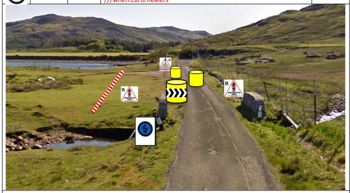
**Spectator area** on R behind fence. ( ///rice.highs.paler) Spectators to stand on rock outcrop, not behind fence. Yellow/black tape – P4A 4.58 0.1 stakes and cones required. Notice D at ends Notice B both sides of road at approx. 10m intervals, Tape gateway on R.
